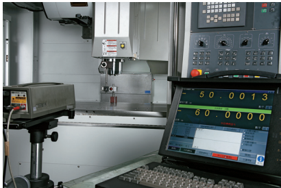
"H.P." laser calibration system ensure machine accuracy & repetition.
